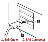
**2.** Connect the SAS cable (1) and power cord (2) to the tape drive.
