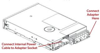
For a SAS drive, connect the power cable of the SAS adapter to the PSU of the server.
