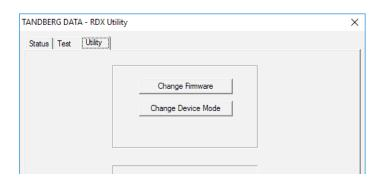
The Change Firmware button can be used to update the firmware if necessary. Click on Change Device Mode.
