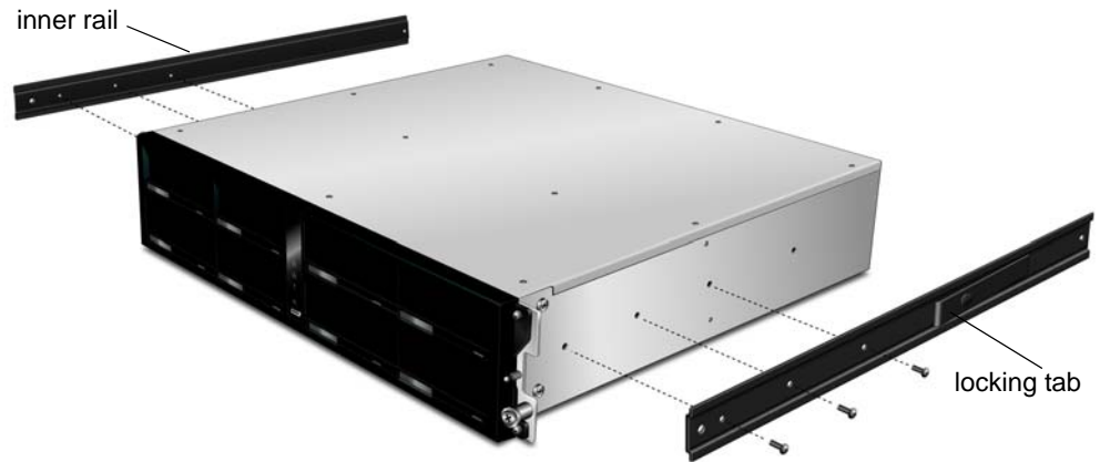
Figure 2-3 Attaching the inner rails to the RDX QuikStation
